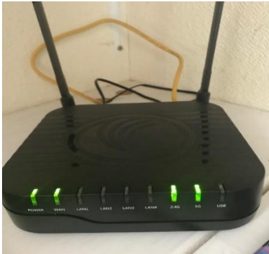
Photograph 1: Correct lights showing. LAN 1-4 will only be illuminated if other devices are plugged in via an ethernet cable.
