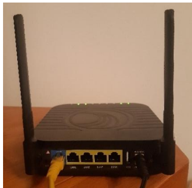
Photograph 2. Yellow cable must be plugged into WAN port (other end into the PoE). Circular black power supply also plugged into AC power adapter.
